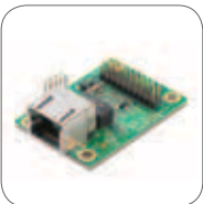
MiiNePort E3 Series PoE pass-through 10/100 Mbps embedded serial device servers
