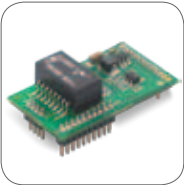
MiiNePort E2 Series Thumb-sized 10/100 Mbps embedded serial device servers
